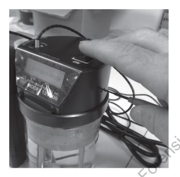
**STEP #3:** Advance first to the final calibration by inserting the small, slotted screwdriver into the mode switch to advance to the display below (press mode switch 2 times to advance to cal adjust screen).
